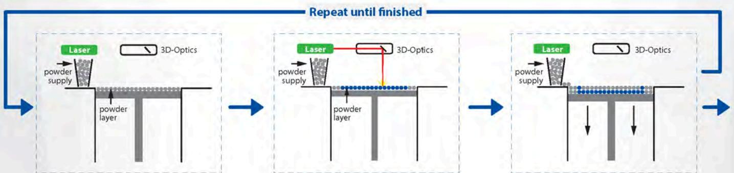
Built on a Windows based user interface, the build job file is loaded onto the machine and the build process constructs the component layer by layer. The build process consists of the cyclical recoating and exposure of the metal powder. This is melted together along the component contours and surface areas defined in pre-processing. Next, the lifting table with the substrate plate is lowered by one layer thickness
